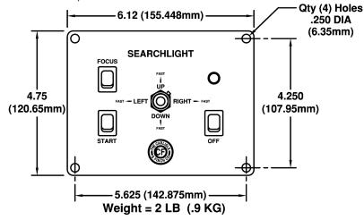
C4-1-1 Master Station.....Depth = 6.5in (166mm) C4-1M-1 and C4E1M-1-2 Secondary.....Depth = 3.5in (89mm)
