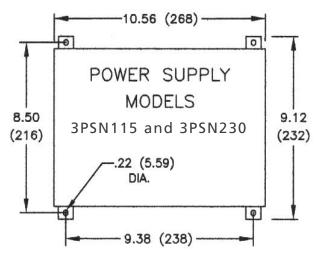
Power Supply 3PSN115 or 3PSN230 Power Supply Weight = 7.5lb (3.4kg)
